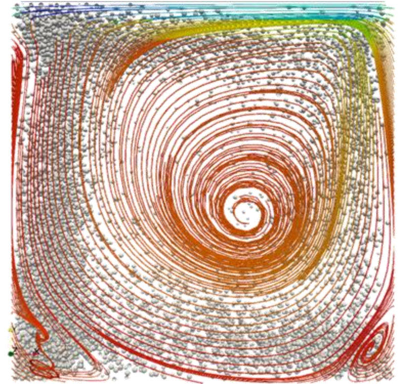
Example of CFD-DEM simulation with OpenFOAM: 50 000 spheres in lid-driven cavity flow.
